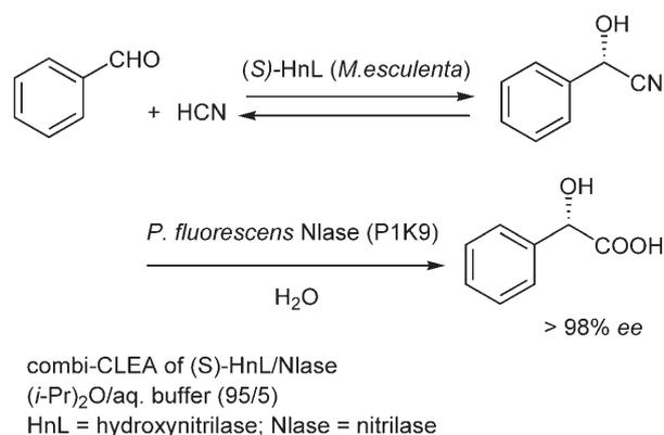
**Figure 17.** One-pot conversion of benzaldehyde to (*S*)-mandelic acid.
