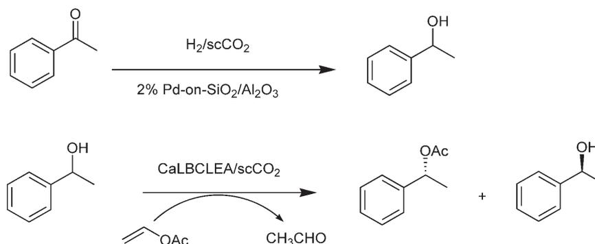
**Figure 15.** Sequential hydrogenation and resolution in  $scCO_2$ .
