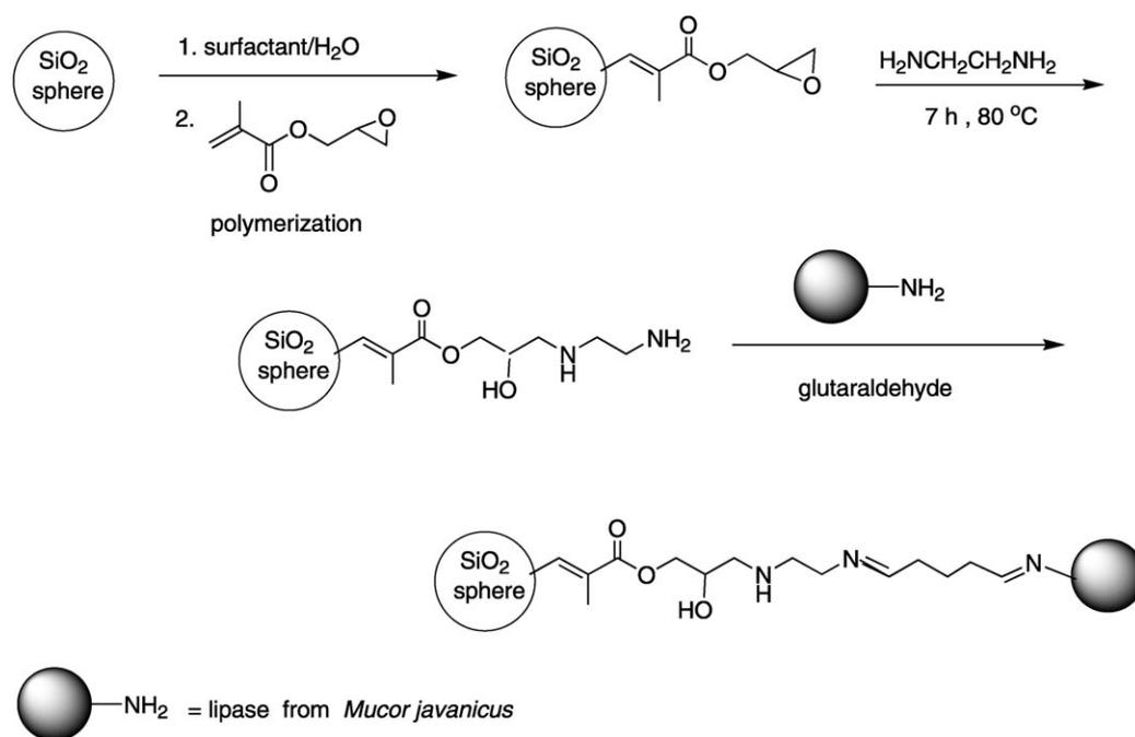
**Figure 6.** Immobilization of a lipase on silica nanoparticles.
