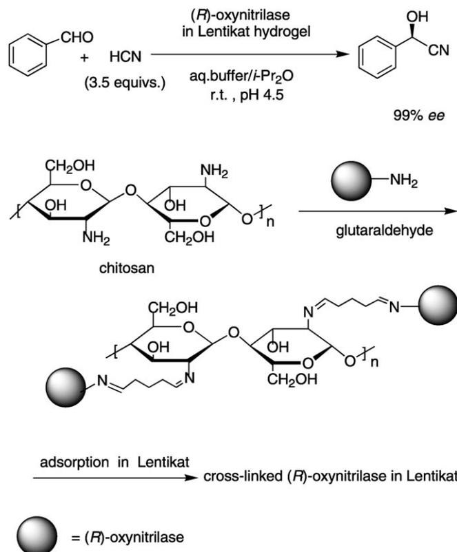
**Figure 4.** Cross-linked (*R*)-oxynitrilase in Lentikat hydrogel.
