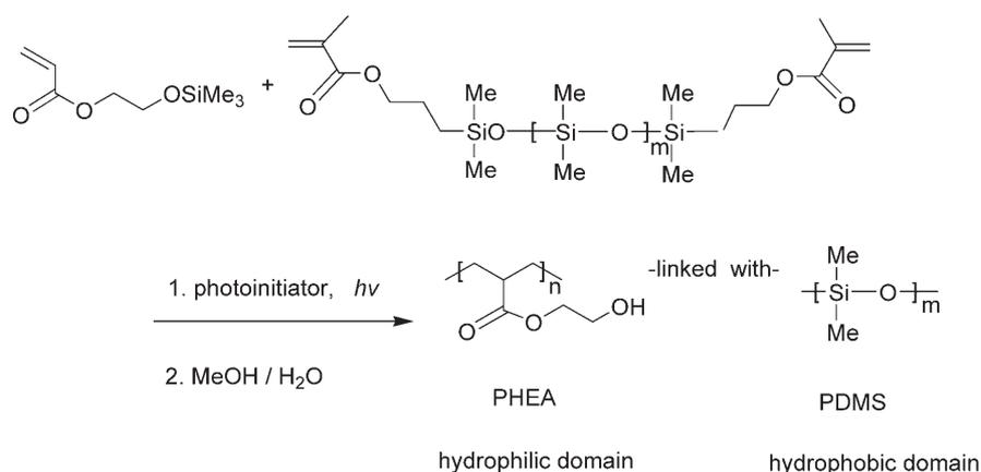
**Figure 5.** Amphiphilic polymer network for enzyme immobilization.
